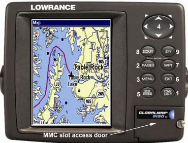
GlobalMap 5150c GPS unit, front view, showing Map Page, keyboard and access door for the MMC slot.
